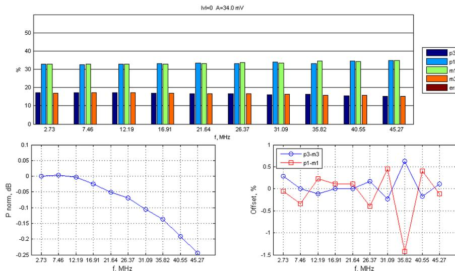
Figure 3: Results of parametrical analysis for sine input signal at different frequencies and amplitude of 34 mV. Threshold №1
