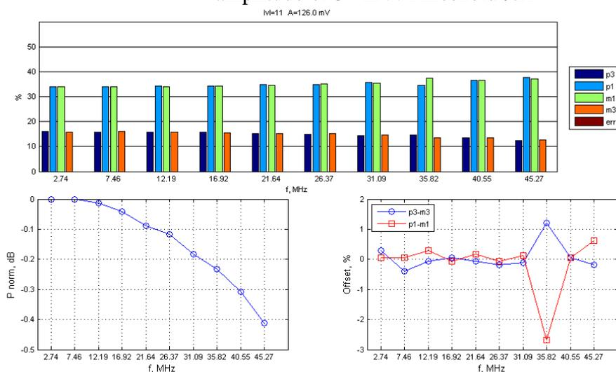
Figure 4: Results of parametrical analysis for sine input signal at different frequencies and amplitude of 126 mV. Threshold №12
