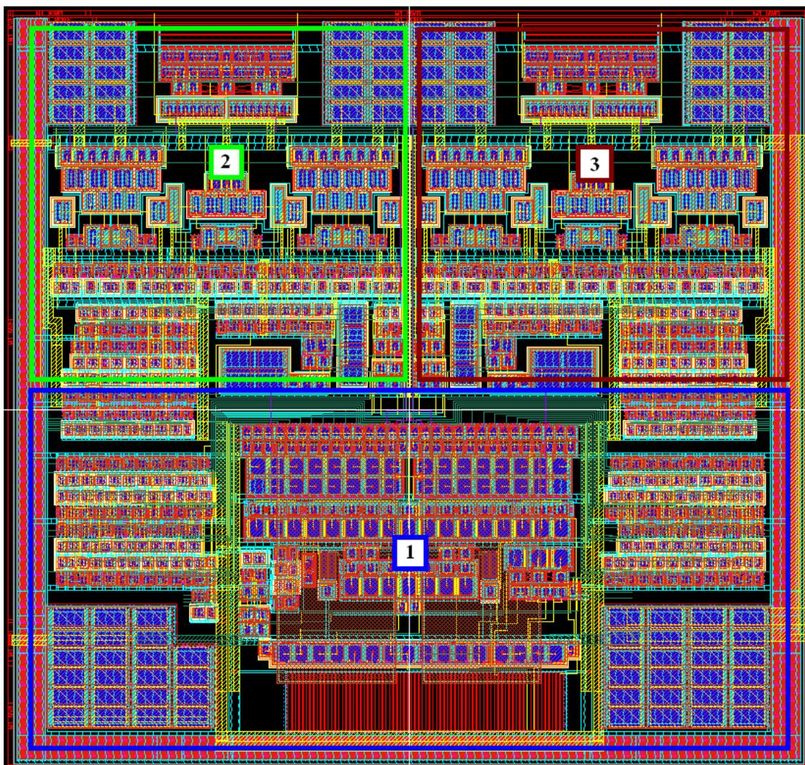
Figure 2: Layout 50 MSPS 2-bit 2-channel special ADC
