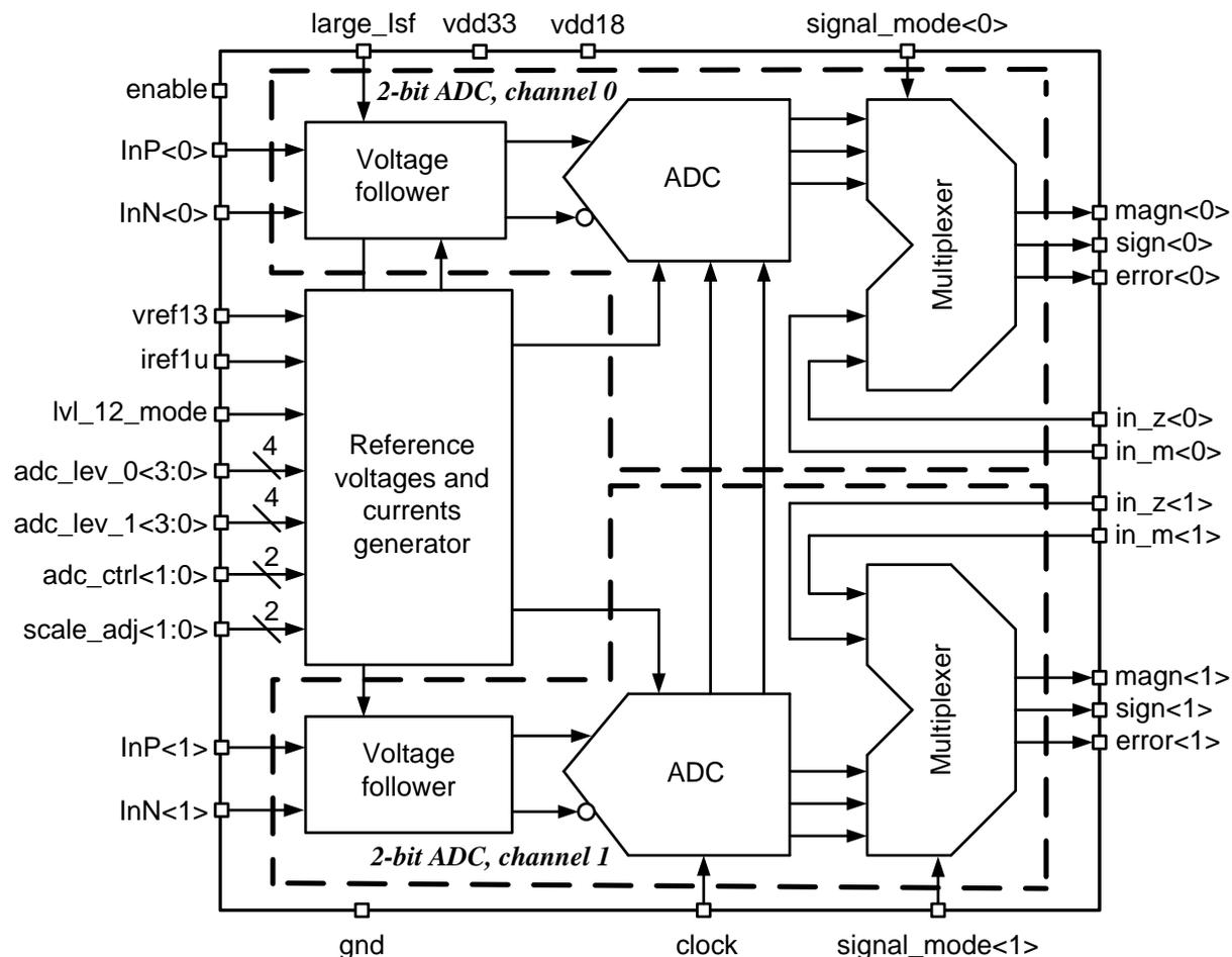
Figure 1: 50 MSPS 2-bit 2-channel special ADC structure
