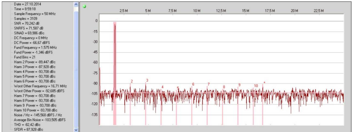
Figure 4: Spectrum, F_s = 50 MSPS, F_{in} = 1.575 MHz
